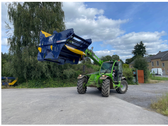
Equipped with a third side, the unroller can also distribute forward.
