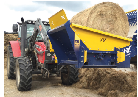
The unroller will take any type of straw, hay or silage bale.
