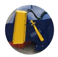
The brush height is manually adjustable on the side of the machine. This allows the height to be adapted depending on the surface or the wear of the brushes.
